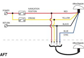
NOT APPROVED FOR INSTALLATION ON CERTIFIED AIRCRAFT THIS IS NOT A TSO/ETSO CERTIFIED LIGHT
