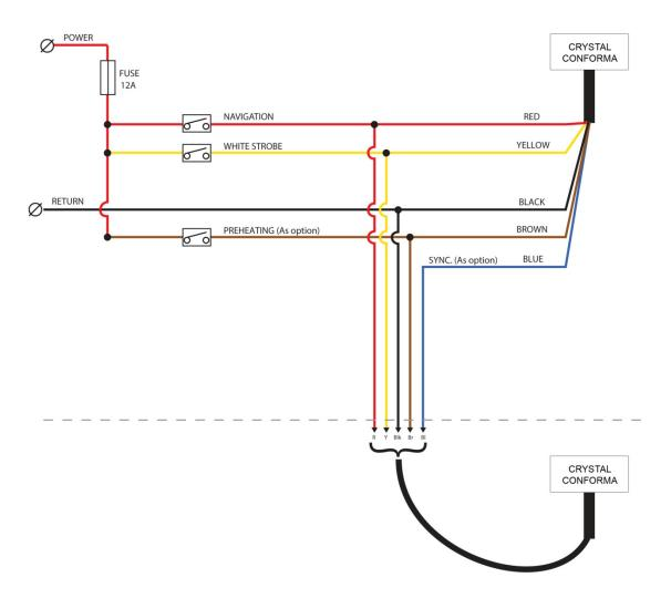
Wire type: multicores 22 AWG, 600 V insulation, 200°C rating;
