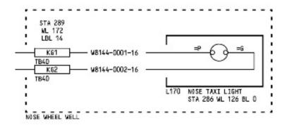
Wiring diagram after installation of Aveo Samson – nose gear taxi light:
