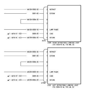
Wiring diagram after installation of Aveo Maximus PowerMax – landing light:
