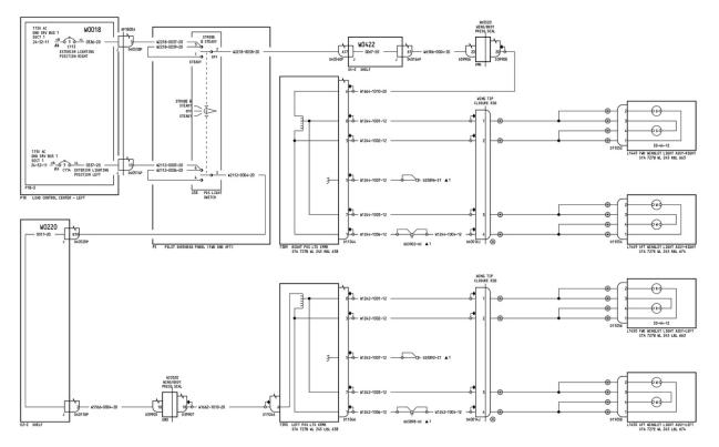
Wiring diagram after installation of Aveo AC/DC converter:
