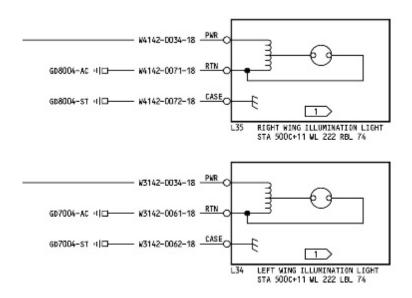
Wiring diagram after installation of Aveo Vesta – wing illumination light:
