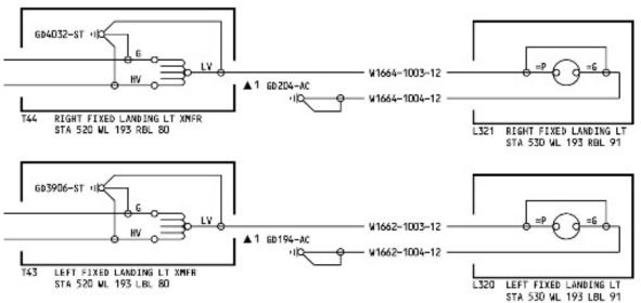
Wiring diagram **after** installation of Aveo Maximus PowerMax – fixed landing light:
