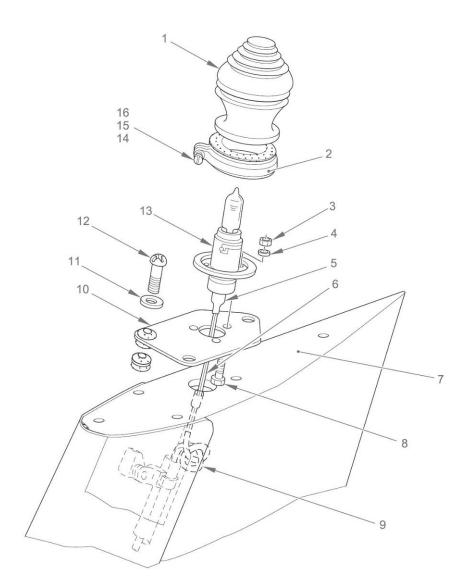
A-2 – Removal of anti-collision light
