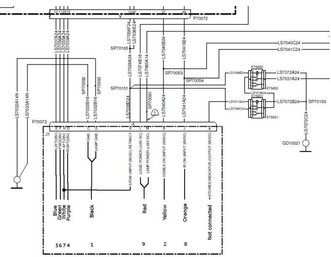
Note: In case of single color light (not dual), there is no orange wire and pin J remains unconnected
