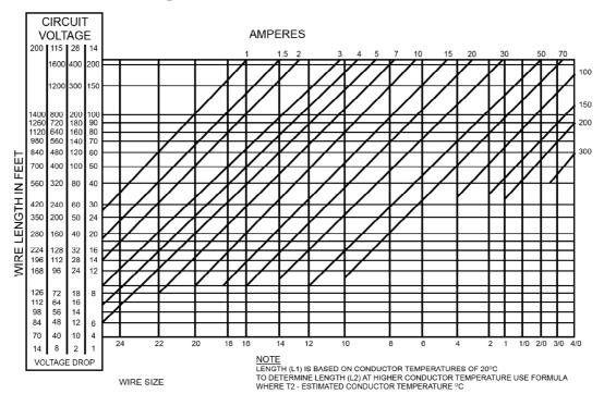
VOLTAGE DROP CHART INTERMITTENT FLOW AT 20° TIN-PLATED MIL-W-27759 CONDUCTOR
