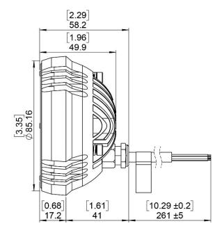
**NOTE:** If the light heats up to the temperature of 85°C (+/-10%), the output drops linearly by up to 10 % from the nominal value until it cools down to 60°C (+/- 10%). As soon as the temperature of 60°C (+/- 10%) is achieved, the light operates at full power again.
