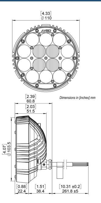
**NOTE:** If the light heats up to the temperature of 85°C (+/-10%), the output drops linearly by up to 10 % from the nominal value until it cools down to 60°C (+/- 10%). As soon as the temperature of 60°C (+/- 10%) is achieved, the light operates at full power again.
