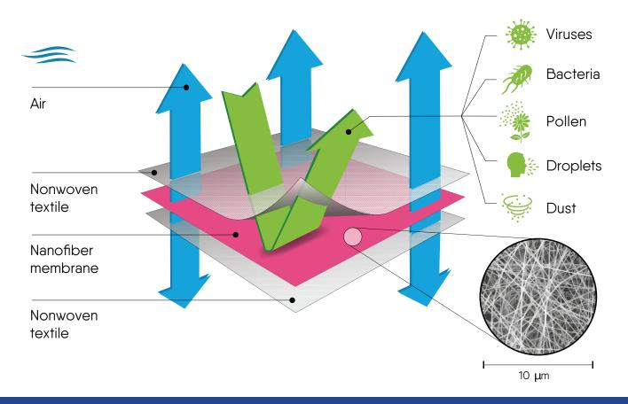
The nanolayer based on a polymer made of PVDF (polyvinylidene fluoride) is formed by a dense netting nanofibers with an average thickness of 50 - 90 nm. Three-layer laminate with nanofiber layer provides high filtration efficiency against various microorganisms, allergens (such as pollen), mold and dust particles with lower pressure slope (resistance to breathing), more precisely with higher breathability of the material, which ensures comfort when breathing.
