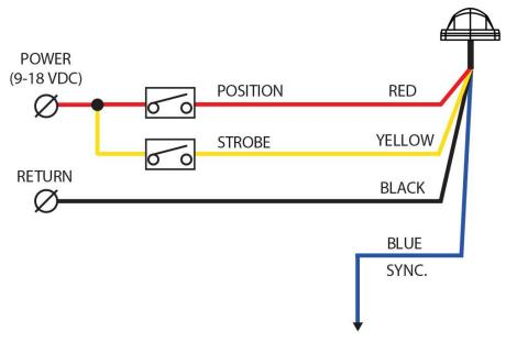
Wire length from base of unit 10.00 inch min.
